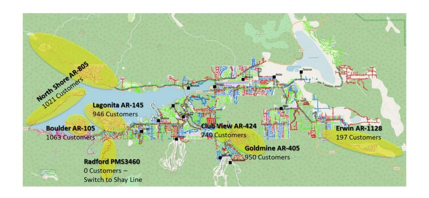
Appendix B: BVES Supply Lines, Sources of Power and Sub-Transmission
